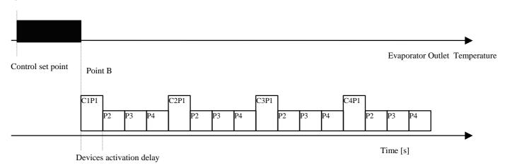
The activation delay of the different devices is the same, without distinction of compressors and capacity control steps.
