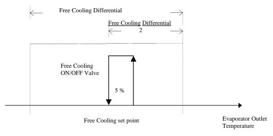
If temperature conditions favour Free Cooling control, the Free Cooling ON/OFF valve will be activated as soon as temperature exceeds the activation threshold of the individual step, identified by a temperature value of:
