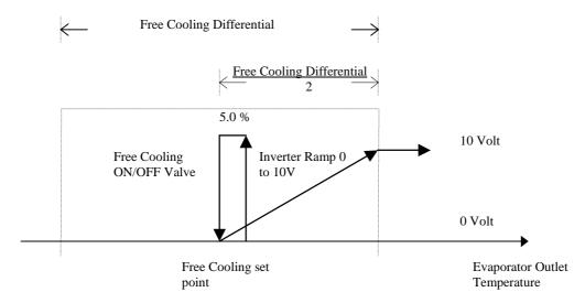
The devices, whether they are valve or fans, will be activated in the second half of the control differential through the effect of the integrating control. Their activation will be tied to the set integrating constant: the slower it is, the greater the value attributed to the specific parameter. The amplitude of the valve control step will be 5.50% of the said control differential.
