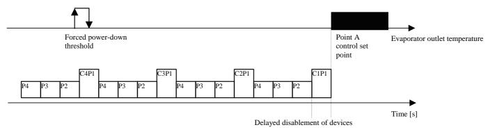
If temperature falls below the set forced power-down threshold, the compressors are powered down irrespective of the set delays, in order to prevent tripping the antifreeze alarm.
