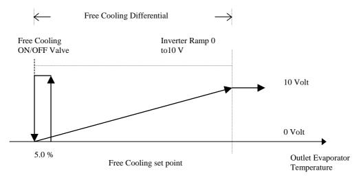
The ON/OFF valve activation step will, in any case, be positioned in the first part of the control differential and will have an amplitude of 5.0% of the said differential.
