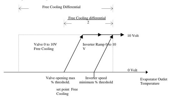
The devices, whether they are valve or fans, will be activated in the second half of the control differential through the effect of the integrating control. This activation will be constrained by the set integrative constant. The greater the value assigned to the integration time, the slower the system's response.
