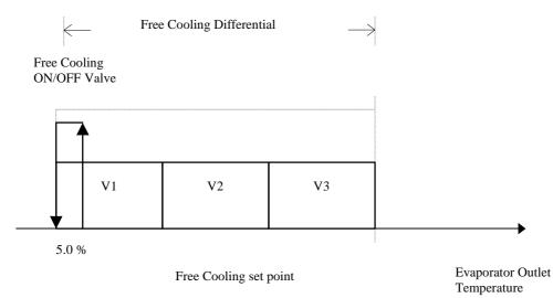
Here is an example of Free Cooling control with ON/OFF valve and three condensation steps.
