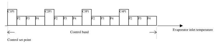
All compressors and the relevant capacity control steps will be proportionally positioned in the band. Increasing temperature values will cause the control steps to be subsequently input. Each step will be input according to the set delay times.
