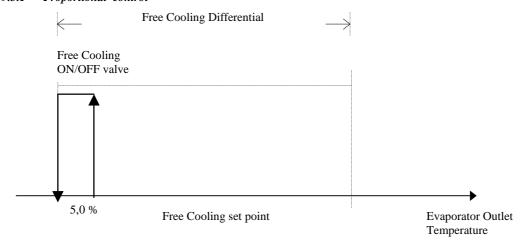
If temperature conditions favour Free Cooling control, the Free Cooling ON/OFF valve will be activated as soon as temperature exceeds the activation threshold of the individual step, identified by a temperature value of:
