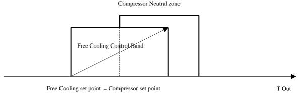
In machines controlled at output with a lateral proportional band, the Free Cooling control set point takes into account an offset with respect to the control set point of the compressors to compensate for the presence of the evaporating battery.
