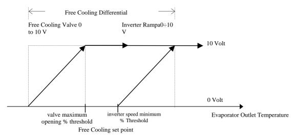
The control proportional ramp of the Free Cooling valve will be calculated inside the area determined by the thresholds:
