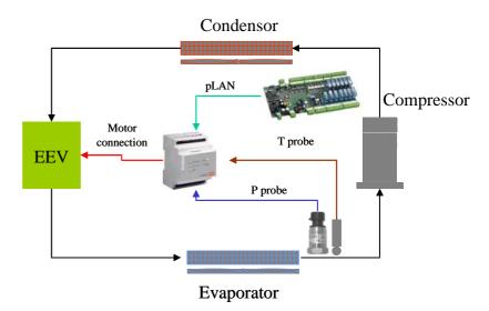
The priorities to be considered for optimal control of the refrigerating system: obtaining a high, constant refrigerating yield rather than very low, stable superheating.
