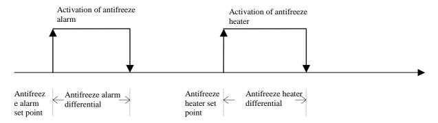
Antifreeze control is always enabled, even if the machine is OFF, both in summer and winter operating modes. For type 5 machines with reversing of the water circuit, the antifreeze control always controls water temperature at evaporator outlet, shifting control to the evaporator or condenser according to the operating mode (summer-winter).
