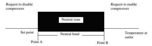
A neutral temperature zone is identified, based on the set set-point and band values.
