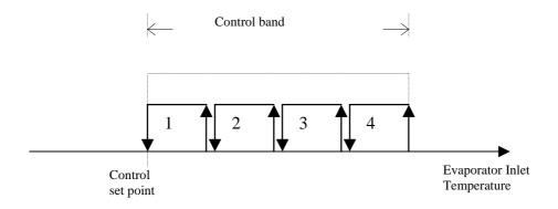
The thermostatic control according to the values measured by the temperature probe at evaporator inlet, is based on proportional control.
