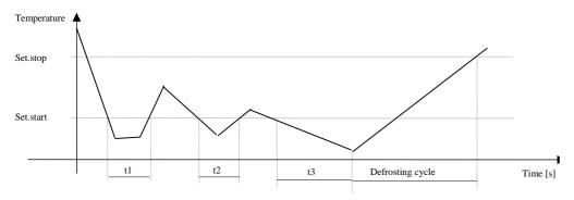
If the battery temperature/pressure remains below the defrosting start set point for a cumulative time equal to defrosting delay time, the circuit in question enters a defrosting cycle.
