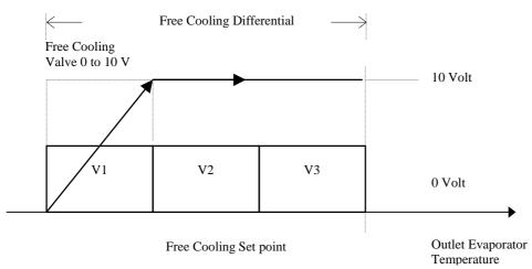
The proportional control ramp of the Free Cooling valve will be calculated inside the first activation step of the condensation fans. In this way, when the first fan is enabled, the valve will be completely open, and, therefore, water flow in the Free Cooling battery (exchanger) will be at maximum level.
