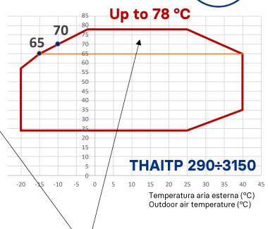
Stable hot water production at 65°C from -15°C to 40°C
